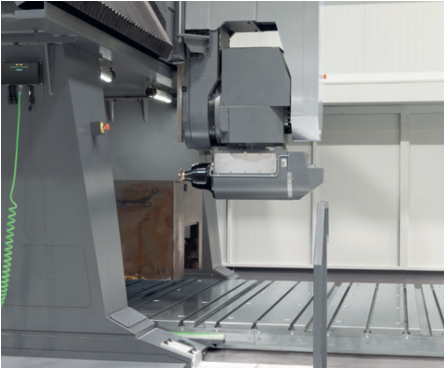
In horizontal spindle position (A-axis tilted by 90°), the long sides and end faces of the workpieces can be machined
