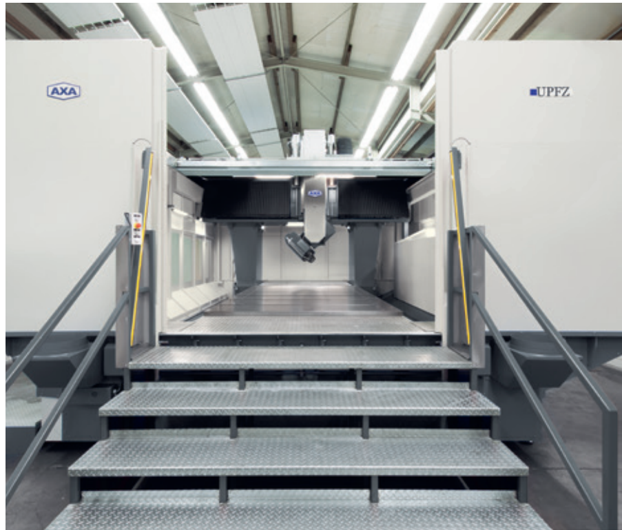
Open roof for loading
