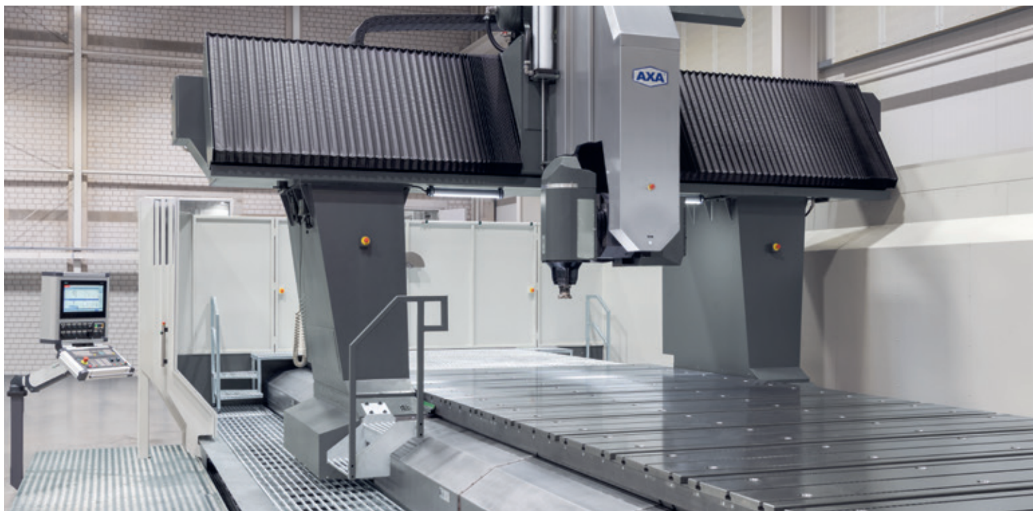
The inclined bed portal reduces the distance between the Y-guideway and the swivel head, thus increasing the overall stability
