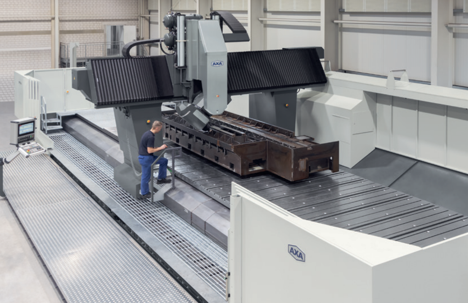
The large gantry machining centre UPFZ: a 2-axis tilting head for 5-side machining of large cubic workpieces
