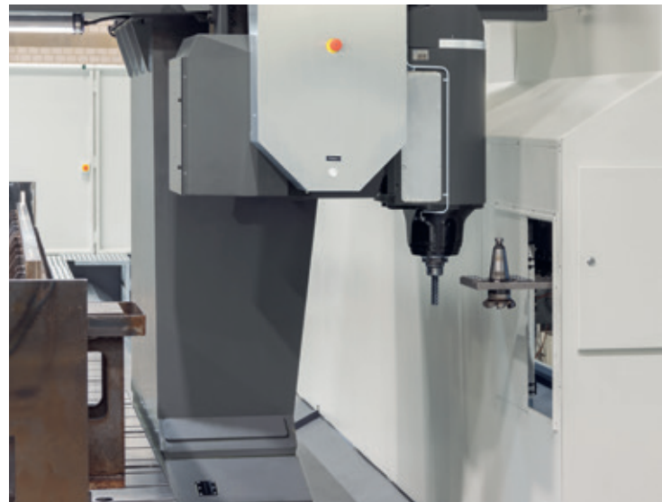
Transfer double gripper with the tool already preselected
