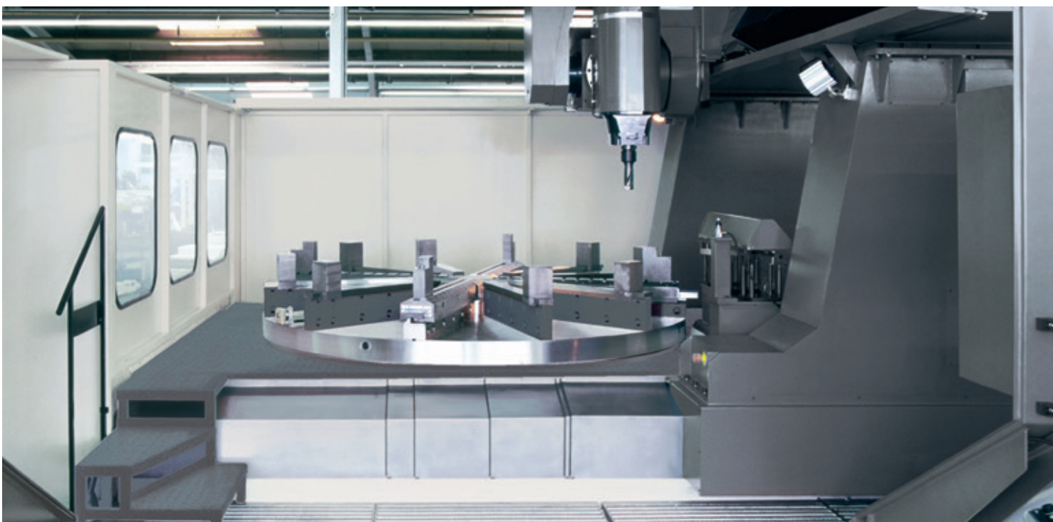
Ring machining with large gantry column machine combined with a rotary table
