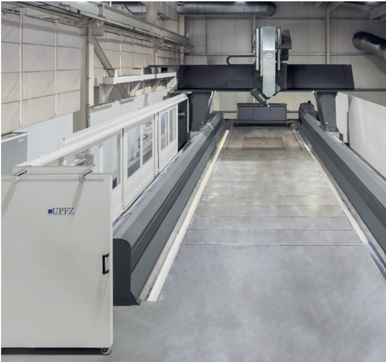
Gantry machining centre UPFZ in special design without machine table and complete covering with front-facing doors
