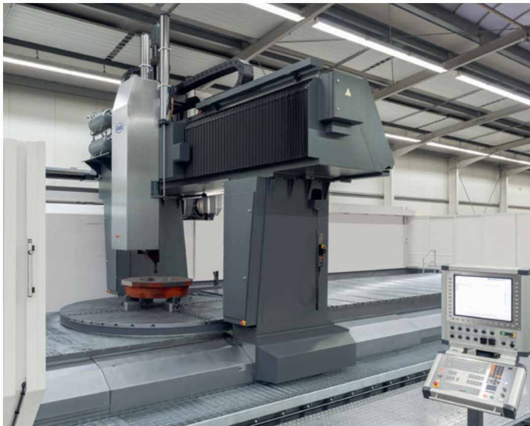
Turning operation: an additional cross support with Y/Z-axis and CAPTO C6 tool holder
