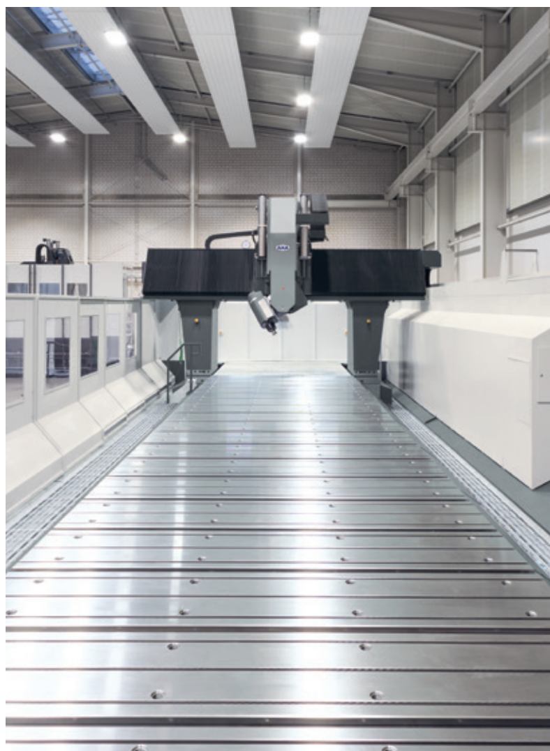
Standard machine tables with integrated T-slots for workpiece clamping
