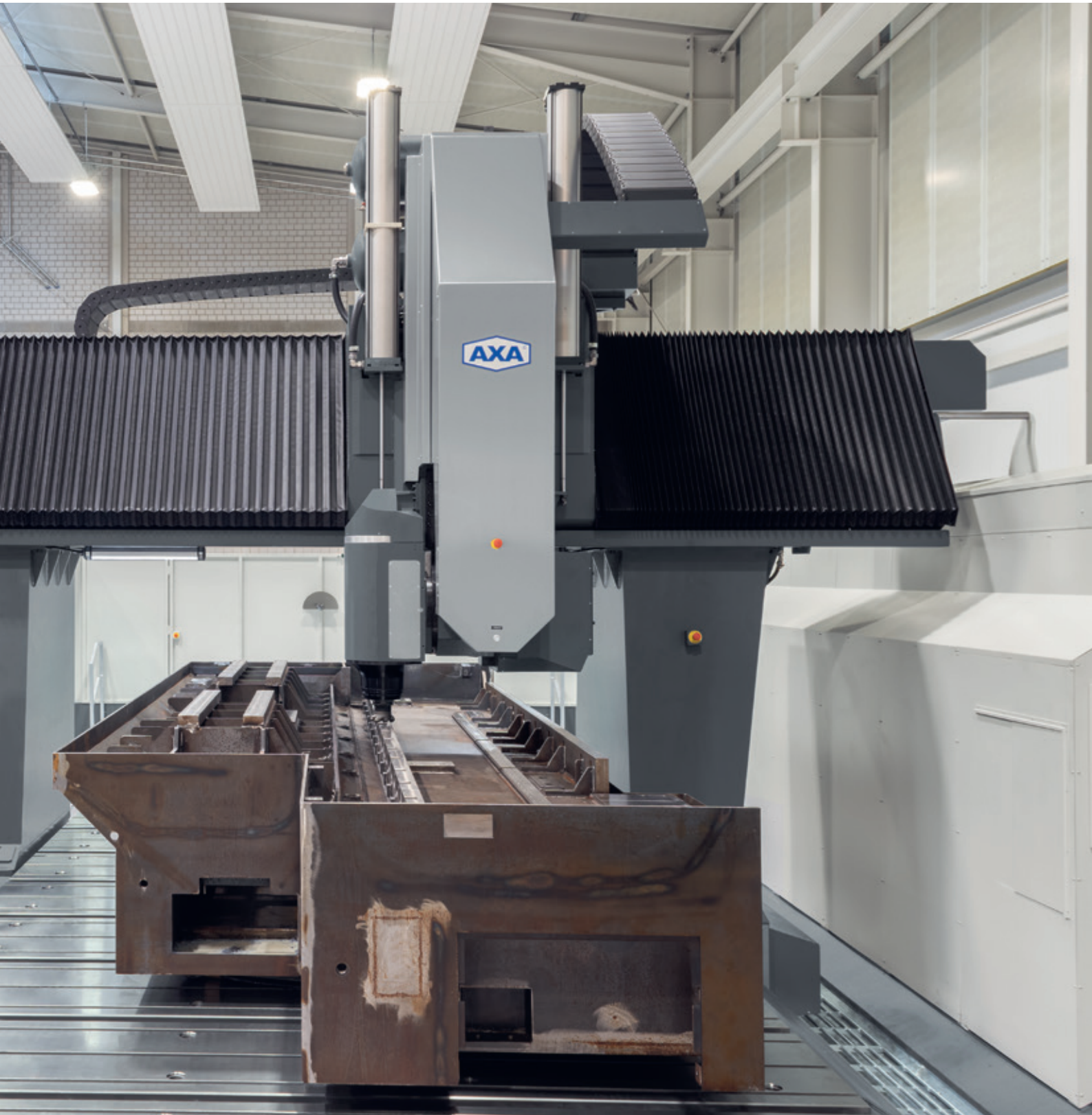
Walk-in work area – perfect accessibility and visibility during set-up and equipping of the machine
