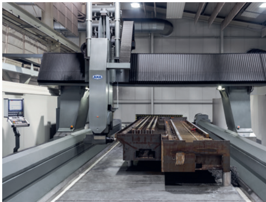
Heavy, solid workpieces are rolled into the machine at ground level – Tie bars with grooves embedded in the floor offer sufficient clamping possibilities
