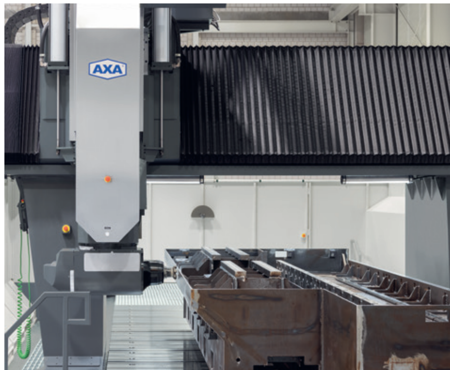
Due to the extended Y-travel path, almost the entire table width is used – an advantage for machining very wide workpieces
