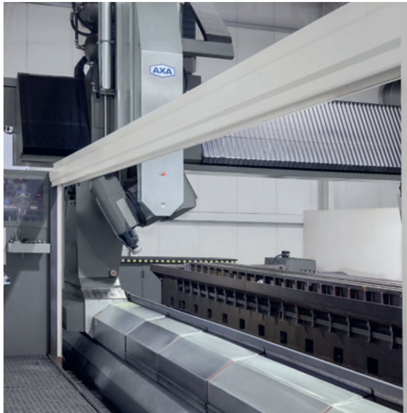
Generous side doors offer good accessibility when setting up the workpieces
