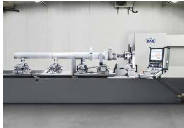
One-sided post-machining of sealing surfaces on long pipes
