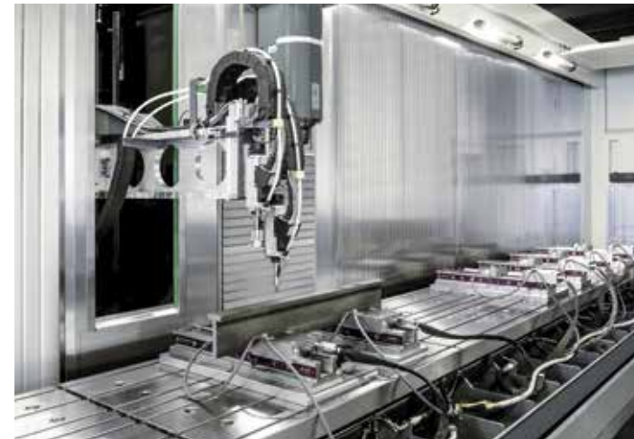
The machining centre with tilting spindle head is used for milling long steel girders and additionally for welding bolts
