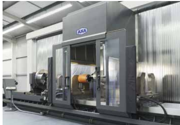
Instead of the fixed machine cladding the working space around the spindle is encased in a hood that moves with the travelling column
