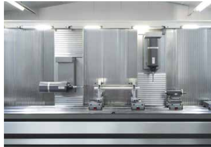
Both spindles can be used in parallel on one workpiece or independently on separate workpieces
