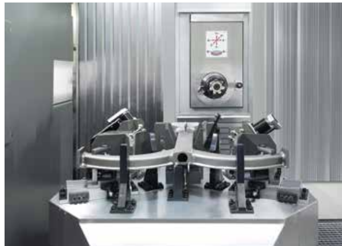
The assembly of the clamping device and workpiece on a rotary table allows several sides to be machined in one clamping operation
