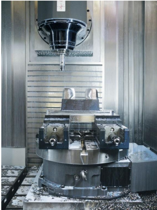
Image 1: Processing a toothed strip on the AXA VCC 50
