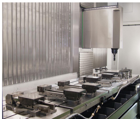
Picture 1: AXA VSC 3 4000 XTS travelling column machining centre– machine table with fixtures for the milling of long parts
