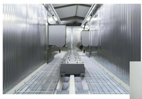
Partial machining from beneath by bolting heavy angular milling heads above a four-point support
