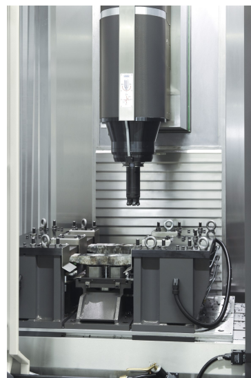
Aligned by means of centring bolts and clamped from beneath against a hydraulically movable surface
