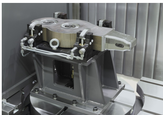
Hydraulically aligned and clamped against impacts
