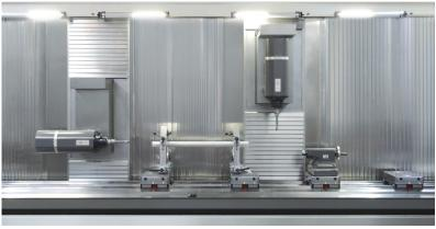
The table area is equipped with guide rails on which support units with rotary tables, clamping shells and tailstocks can be flexibly fitted and positioned.
