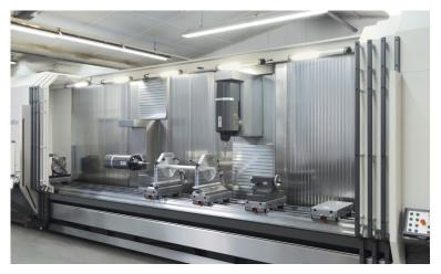
Using the rotary table and tailstock, the workpiece can be rotated in position in addition to the tilting spindle heads.
