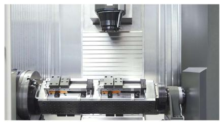
On the swivelling bridge installed in the left-hand pendulum working space, several workpieces can be clamped in parallel and each machined on three sides
