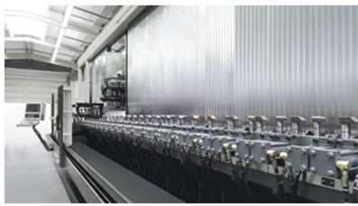
The clamping elements each open and pivot sideways to uncover the area to be machined for the milling tool as it moves past.
